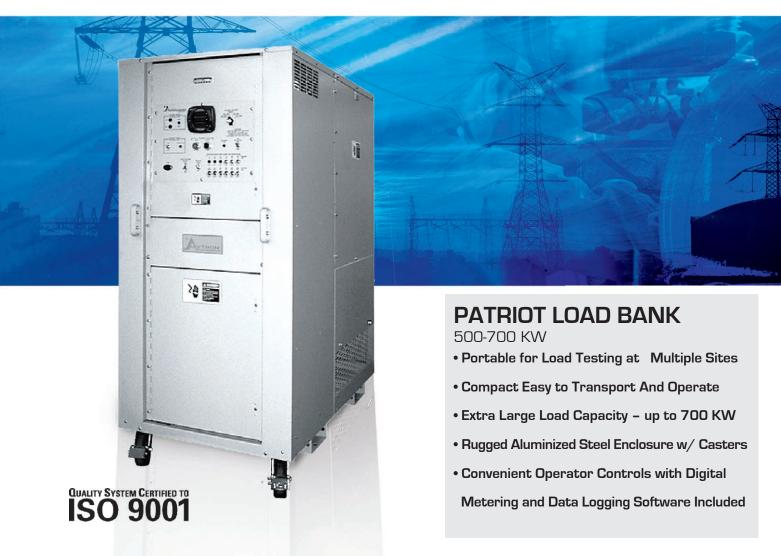
The Avtron Patriot Load Bank is a portable, self-contained unit that simulates electrical loads. It is ideal for routine load testing of standby diesel generating systems at remote sites or for factory production line testing of (UPS) Uninterruptible Power Supplies, turbines, or engine generator sets. This model provides resistive loading up to 700 KW at either 240/480 Volts AC in a convenient, and easy - to - use package.
